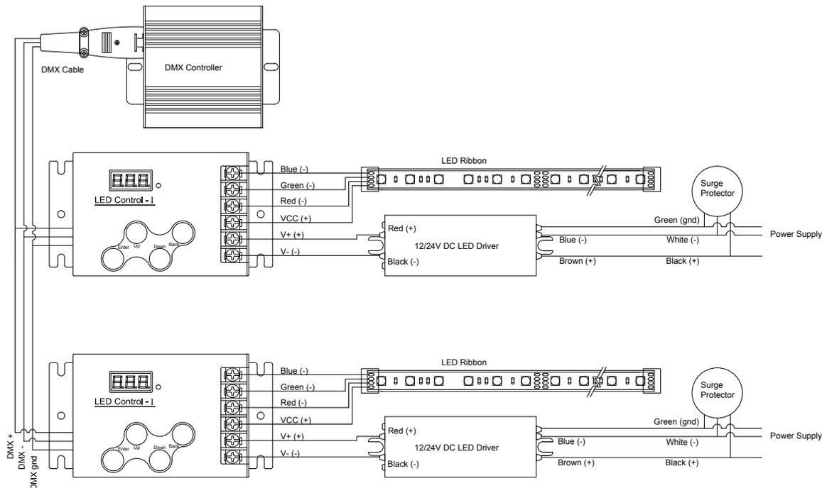
RGB LED Ribbon with T80 Controller and Amplifier
