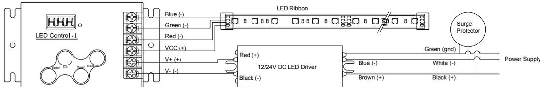
RGB LED Ribbon with LCI Controller to DMX Master controller
