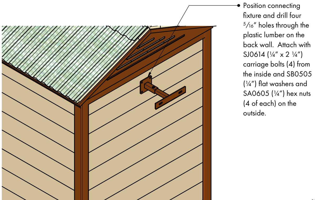
**16** Attach the vent stack to the outhouse and secure using the U-bolt.
