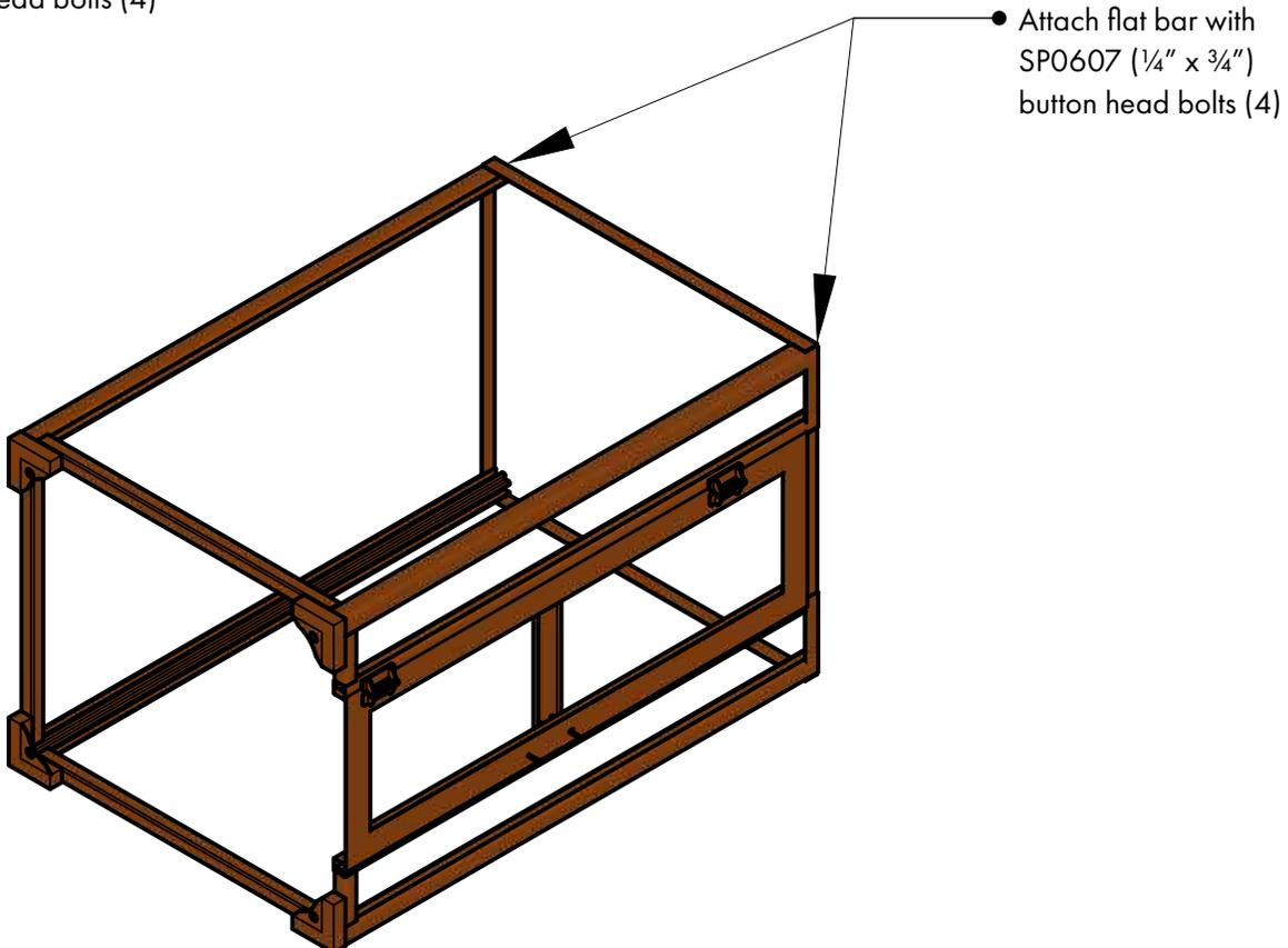
Attach flat bar with SP0607 (1/4" x 3/4") button head bolts (4)
