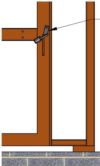
• Keep the locking bolt for use in decommissioning the outhouse with an appropriate padlock
