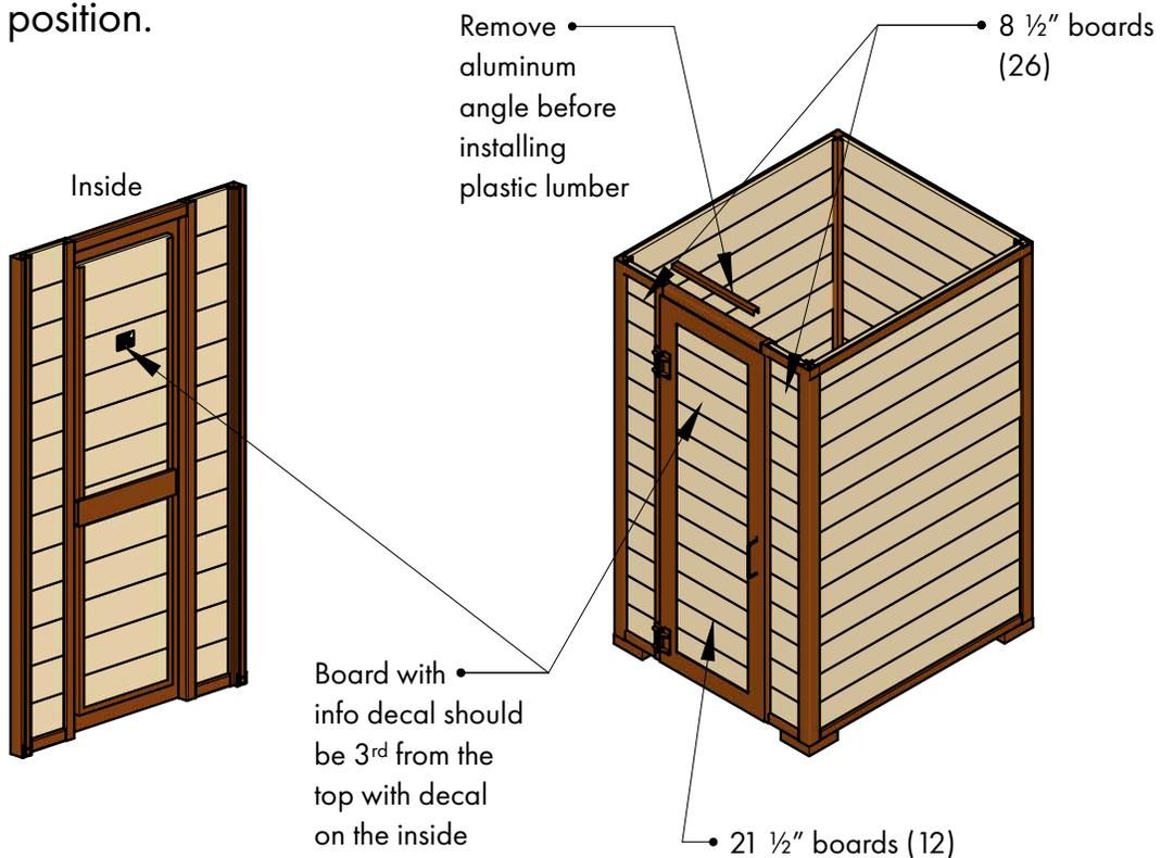
**11** Re-install the aluminum angle back above the top board on the door.
