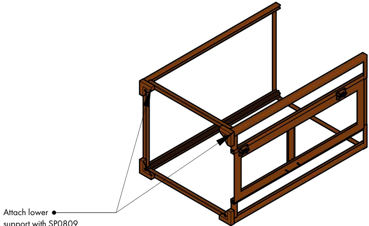
Attach lower support with SP0809 (3/8" x 1") button head bolts (4)
