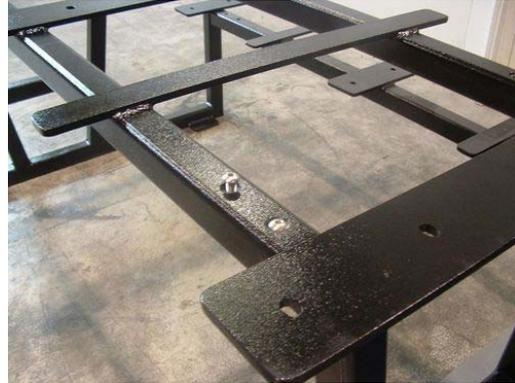
4. Lay the plastic boards on the table with predrilled countersunk holes facing upwards and drop in tapered head bolts.
