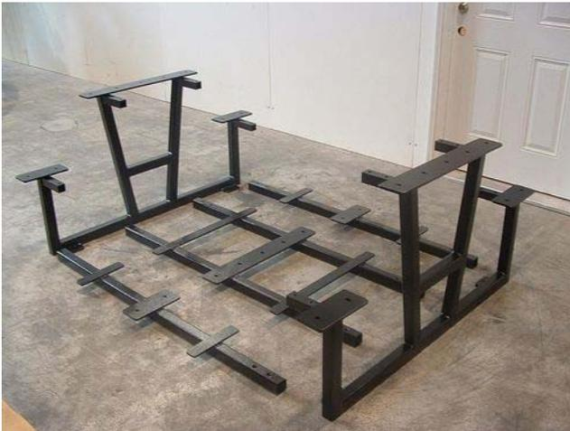
2. Insert the leg and seat supports into the receiving extensions of the leg ends.
