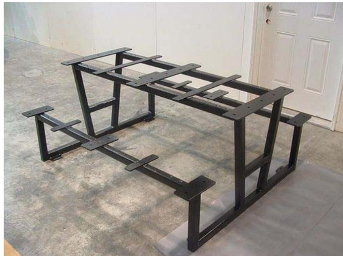
3. Put **LOCTITE®** Threadlocker super glue on 1-1/2" button head bolts and secure leg and seat supports. If supports have 2 holes, only one bolt is necessary. DO NOT OVER TIGHTEN. DO NOT CROSS THREAD.
